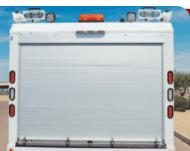
▼ Extruded doublesided aluminum slats are easily replaced in case of damage. End caps are removable.
